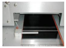
Installed sensor with quartz rod to pick up UV energy.
